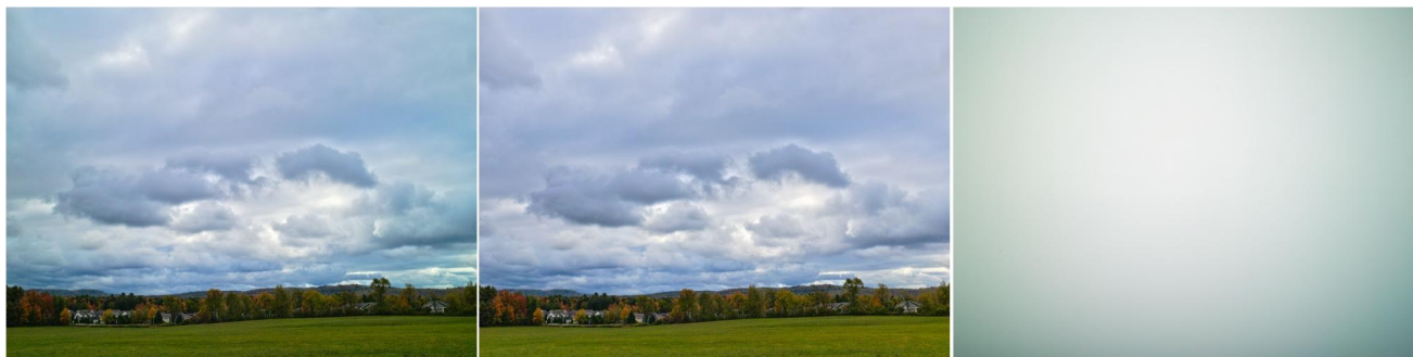
Example of the flat field correction. Image before, image after correction and the flat field file used. Notice the correction of both luminosity and color non-uniformities.
